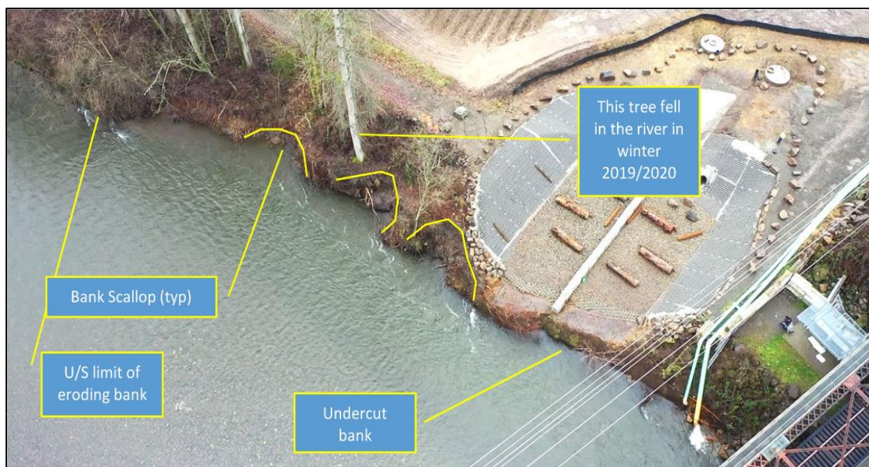
Figure 4-20. December 2019 UAV image annotated with erosional features. The riverbank shown above waterward of the edge of outfall has slumped or eroded back 5-10 feet since this photo was taken.
