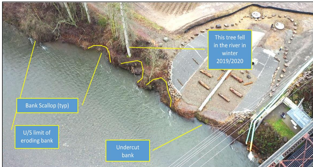
Figure 4-10. December 2019 UAV image annotated with erosional features. The riverbank waterward of the edge of outfall has eroded 5–10 feet since this photo was taken.
